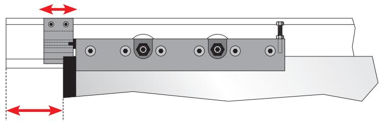
**9 Aushebelschutz justieren**
